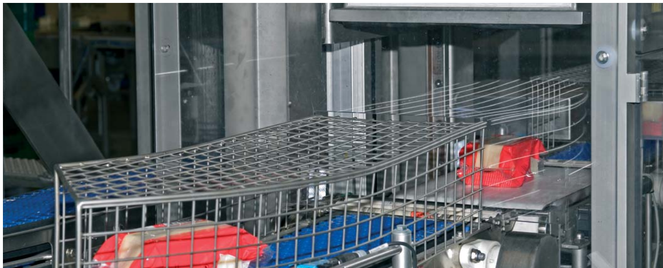
Individual packages are returned to the production line when they have passed the CO 2 leak test in LeakMatic.
