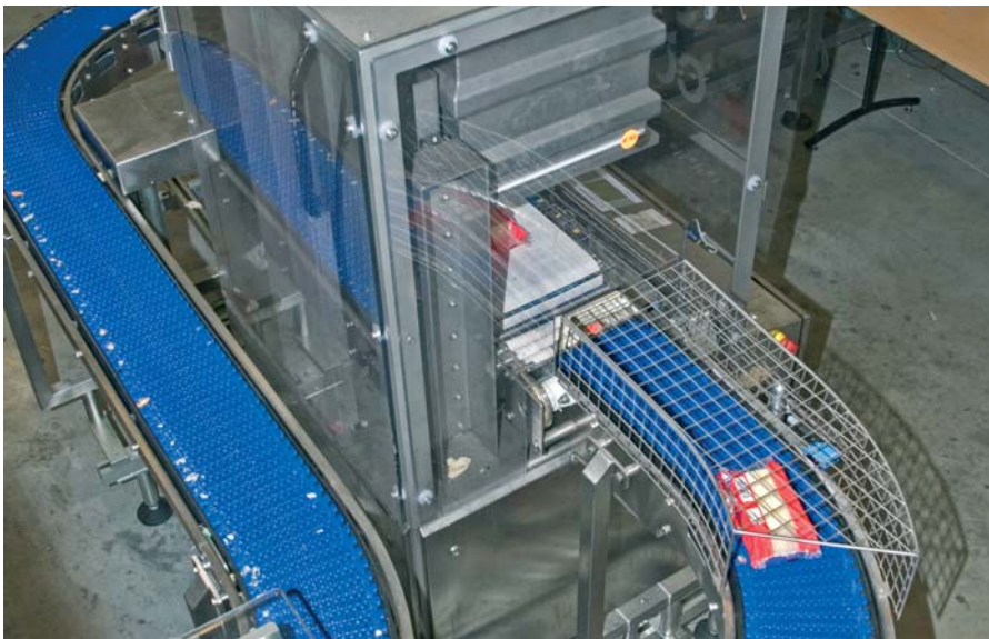
Packages are tested on a parallel conveyor containing LeakMatic.
